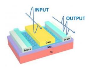
Graphene transistor. Image credit: Peking University
