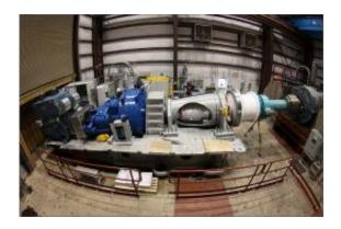
A coupling of giants: Samsung's 2.5-megawatt wind turbine drive train meets the National Wind Technology Center's 2.5-megawatt dynamometer. Samsung's drive train weighs 90 tons and is the brains behind its 2.5-megawatt wind turbine that can supply electricity to 1,800 homes. Credit: Rob Wallen
