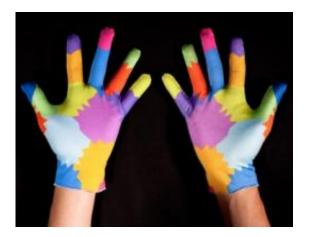
The hardware for a new gesture-based computing system consists of nothing more than an ordinary webcam and a pair of brightly colored lycra gloves. Photo: Jason Dorfman/CSAIL
