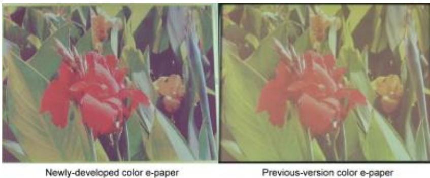
Figure 1: Display image comparison of Fujitsu's new version vs. previous-version color e-paper
