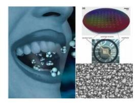
Exhaled air from diabetics contains slightly higher levels of acetone vapor than healthy persons. A new kind of sensor can now selectively detect acetone even in the smallest concentrations.
