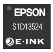
Seiko Epson and E Ink Corporation today announced a new jointly developed display controller IC. The S1D13524 is a high-performance EPD controller with a built-in color processor for E Ink's VizplexTM-enabled electronic color paper displays. Targeting color and very high resolution B&W applications, the new IC is based on the same powerful engine as the first two models, the S1D13521 and the S1D13522, but also includes a color processor that allows simple customization.
