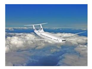
MIT's D "double bubble" series design concept is based on a modified "tube-andwing" structure that has a very wide fuselage to provide extra lift. The aircraft would be used for domestic flights to carry 180 passengers in a coach cabin roomier than that of a Boeing 737-800. Image: MIT/Aurora Flight Sciences
