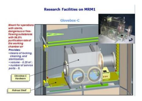
Glovebox-C is intended for operations with sterile, dangerous or free-flowing substances, providing a 99,9% purification rate of the working chamber air. Image credit: S.P. Korolev Rocket and Space Corporation Energia
