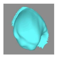
This three-dimensional scan of the ear canal, taken with new imaging technology developed at MIT, could be used to manufacture better fitting hearing aids. Image: Federico Frigerio
