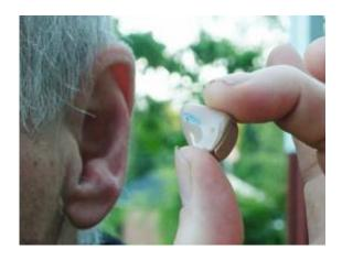
Hearing aids work best when there is a tight seal between the device and the wearer's ear canal.
