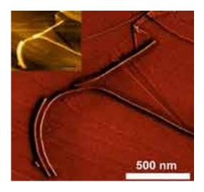
Cylindrical nanostructures on a carbon surface.
