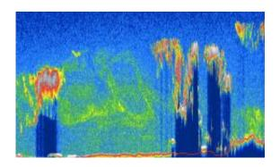
The six-mile-high Chinese dust plume detected by CALIPSO appears as yellow-green swirls in this image. The tall columns topped in red and yellow are clouds. Credit: NASA
