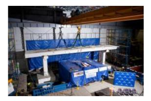
The UB seismic test on a 70-ton bridge specimen may lead to more costeffective methods of building bridges in earthquake-prone areas, like California.
