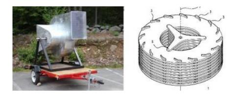
(Left) The bladeless wind turbine, and (right) the stack of disks which rotate and are connected to a shaft. Image credit: Solar Aero.
