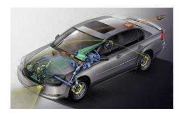
GMC's Yukon hybrid, control software logic analyzes hundreds of inputs every 10 milliseconds, including vehicle load, engine operations, battery parameters, and the temperatures in the high-voltage electric components. Credit: GMC
