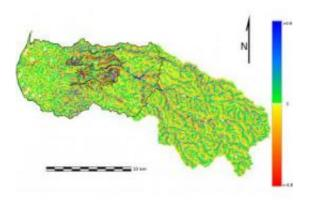
Map of modeled cumulative hillslope erosion/deposition (HED) for the Wadi Ziqlab watershed after 200 years. The map shows HED due to human landuse, after subtracting 'natural' surface change from surface change with shifting cultivation and grazing. Credit: The Mediterranean Landscape Dynamics Project/ASU/NSF
