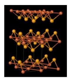
The crystalline structure of the superconductor FeSe has square layers of iron (Fe) atoms that are strongly chemically bonded to layers of selenium (Se) atoms. The superconducting electrons are found in the iron layers. The group's work showed that a deviation of the shape of the iron layers from exactly square geometry at the length scale of thousands of atoms is a critical factor in determining whether superconductivity occurs or doesn't occur.
