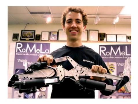
Derek Lahr, a Ph.D. student at RoMeLa, holds the leg of the humanoid robot, CHARLI H. This bulky, stronger robot will utilize various technologies that may allow it to walk outside.
