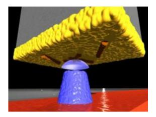
In this diagram, viruses (colored orange) cling to the gold surface (yellow) at the end of a silicon cantilever. A magnetic tip (blue) creates a magnetic field that interacts with the viruses to create an image, using magnetic force resonance microscopy. Image: Martino Poggio, University of Basel
