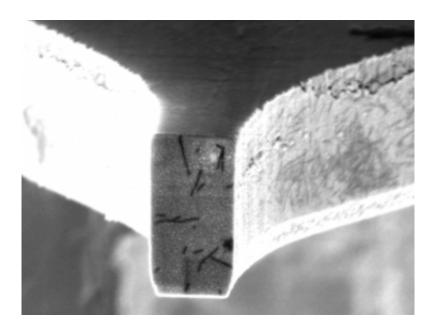
An electron micrograph showing the tip of the cantilever, with virus particles attached. Image: Christian Degen
