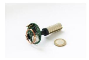
The passive sensor-transponder continuously monitors the protective coating of concrete bridges, allowing corrosion damage to be detected at an early stage. ( $\bigcirc$  Fraunhofer IMS)
