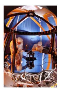
Engineers at Ball Aerospace test the Wavefront Sensing and Control testbed to ensure that the 18 primary mirror segments and one secondary mirror on JWST work as one. The test is performed on a 1/6 scale model of the JWST mirrors. Credit: NASA/Northrop Grumman/Ball Aerospace
