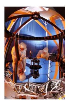
Engineers at Ball Aerospace test the Wavefront Sensing and Control testbed to ensure that the 18 primary mirror segments and one secondary mirror on JWST work as one. The test is performed on a 1/6 scale model of the JWST mirrors. Credit: NASA/Northrop Grumman/Ball Aerospace
