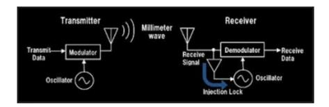
Injection lock system is used in the receiver to synchronize it to the transmitter frequency. This eliminates the need for phase-lock loop system that uses more power and takes up additional space. Credit: Sony Corp.
