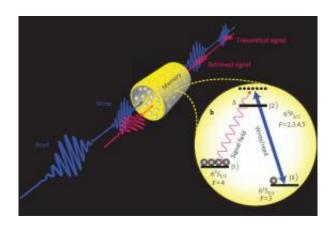
In the optical quantum memory, a signal containing the information and a write pulse are sent together into a cesium vapor cell. The vapor turns the pulses into a spin wave, and the information can be retrieved by a read pulse that converts the spin wave into an optical signal. The memory can achieve data rates that exceed 1 GHz. Image copyright: K.F. Reim, et al.
