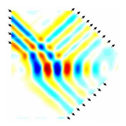
Image from laboratory experiment on internal waves shows both reflection and transmission of waves through a boundary between layers of water with differing densities
