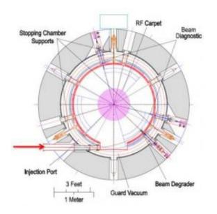
A reverse-cyclotron will help trap high-speed particles in a plasma soup. Credit: Michigan State University
