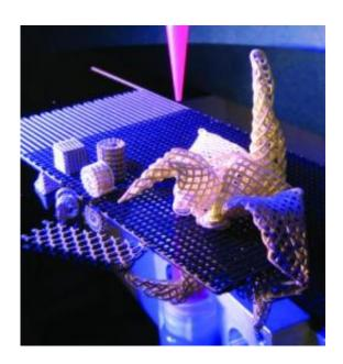
These structures were folded from flat sheets of direct-printed titanium hydride ink, a new technique pioneered by University of Illinois researchers. Credit: Bok Yoep Ahn
