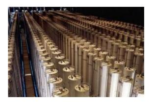
Gas centrifuge plants that enrich uranium — such as this one in Piketon, Ohio — are large and hard to hide. A new laser process would make enrichment possible on a cheaper, smaller scale, upping the potential for nuclear proliferation.
