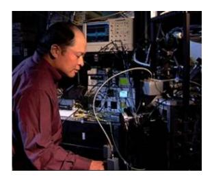
NIST physicist Sae Woo Nam works with refrigeration equipment used to cool photon detectors to nearly absolute zero. His team's efforts have created devices that can detect single photons with 99 percent efficiency. Credit: NIST
