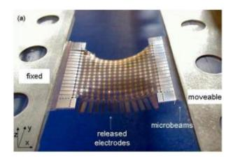
A network with 256 micronodes (gold dots) is stretched in the hand-controlled stretching device. After being stretched in one direction, the network is rotated 90° and stretched in the other direction. Image credit: G. Lanzara, et al.
