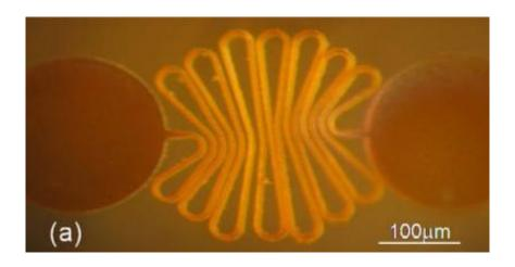
Two micronodes are connected by a microwire that is arranged into loops and segments to enable low-strain stretching. Image credit: G. Lanzara, et al.
