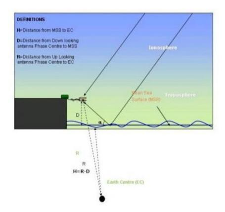
Oceanpal is Star2Earth response to sea and lake surface monitoring. It is a passive system using any available signals from navigation satellites such as GPS, EGNOS and future Galileo to deliver information about surface height and surface state. The above figure illustrates the Oceanpal principle of measuring direct and indirect navigation satellite signals. Credits: Star2Earth
