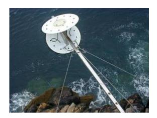
Star2Earth's Oceanpal sensor installed on water front for measuring of water levels and wave heights. Credits: Star2Earth
