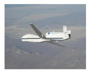
The Global Hawk can fly autonomously to altitudes above 60,000 feet -- roughly twice as high as a commercial airliner -- and as far as 11,000 nautical miles. Operators pre-program a flight path, and then the plane flies itself for as long as 30 hours. Credit: NASA/Dryden/Carla Thomas
