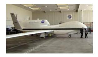
A NASA Global Hawk robotic jet sits in a hangar at Dryden Flight Research Center in Edwards Air Force Base, Calif., on April 13, 2010. The Air Force turned over to NASA three Global Hawks, which were designed for military reconnaissance but equipped with science sensors for conducting atmospheric research over the Pacific. The space agency will use them for unmanned, long-duration, autonomous research flights.(AP Photo/John Antczak)
