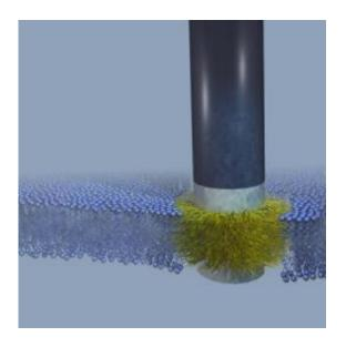
A "stealth" probe sits firmly fused into a cell membrane. The membrane is represented by the small blue spheres, with the hydrophobic portion inside shown by squiggly fine blue lines. The silicon part of the probe is black and the chromium bands that bound the thin gold band are silver-gray. The gold band is obscured by the carbon atoms that are attached to it and that integrate with the hydrophobic part of the membrane. Credit: Benjamin Almquist, Stanford University
