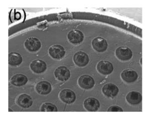
Nanotubes grown in holes in silicon dioxide wafers have the potential to outperform currently available filters for many uses, Rice researchers found.
