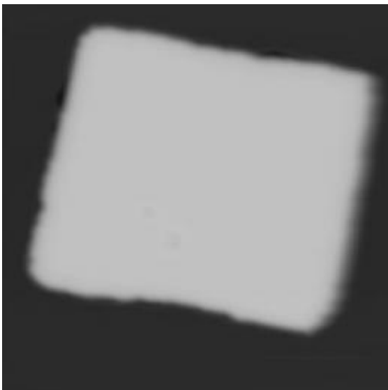
Figure 1: STM image of ultrathin MgO film on Ag(100) surface.
