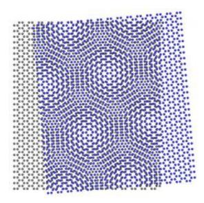
Moiré patterns appear when two or more periodic grids are overlaid slightly askew, which creates a new larger periodic pattern. Researchers from NIST and Georgia Tech imaged and interpreted the moiré patterns created by overlaid sheets of graphene to determine how the lattices of the individual sheets were stacked in relation to one another and to find subtle strains in the regions of bulges or wrinkles in the sheets. Credit: NIST
