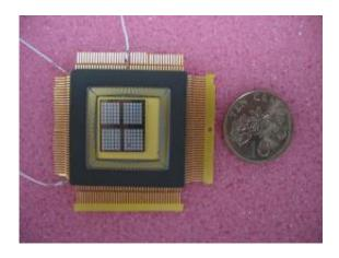
A prototype of the thermoelectric power generator assembled in a ceramic package and placed next to a Singapore ten-cent coin. Image credit: Jin Xie, et al.
