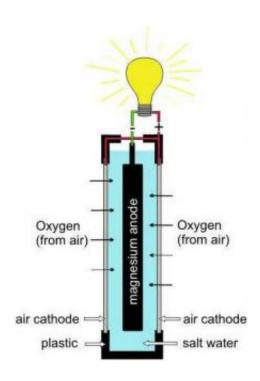
Magnesium + Oxygen + Water + Salt + Additive = Direct Current Credit: MagPower Systems, Inc
