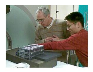
Zachary Levine (at left) and Joe Chen prepare to load a boxful of polymer ellipsoids into a CT scanner to test its ability to measure lung tumors' volumes.
