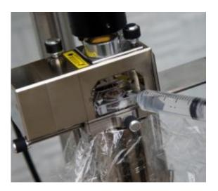
An Atomic Force Microscope, which is used to capture high-resolution images of liquid-solid interfaces. Photo: Patrick Gillooly
