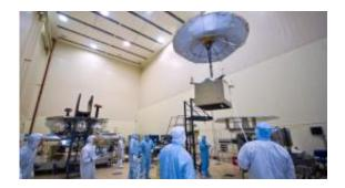
Workers move into place the vault that will protect Juno's sensitive electronics from Jupiter's intense radiation belts. Image credit: NASA/JPL/Lockheed Martin
