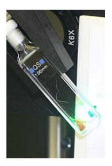
Ultraviolet light breaks down a chemical agent inside a quartz cuvette. The brown material is the decomposition byproduct.
