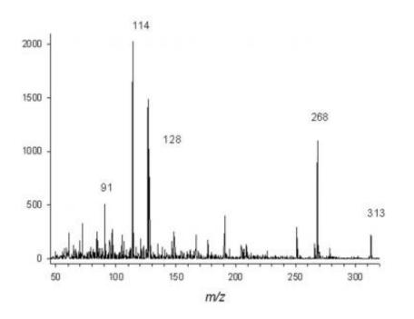
A mass spectrometry reading shows that laser light degraded the nerve agent VX (spike at 268) into two harmless daughter products (spikes at 114 and 128).
