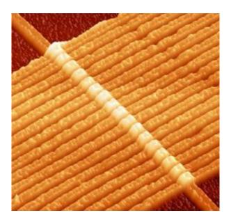
An image of a circuit with 17 memristors captured by an atomic force microscope. Each memristor is composed of two layers of titanium dioxide connected by wire. As electrical current is applied to one layer, the small signal resistance of the other layer is changed, which may in turn be used as a method to register data.
