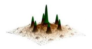
A residual interaction with the SiC substrate causes the formation of the six-fold satellite reflex structure. Credit: Source: Christoph Tegenkamp, Leibniz University Hanover
