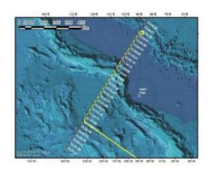
On 20 April 2010, NASA flew a DC-8 directly under CryoSat-2 orbiting above. The DC-8 flight trajectory is marked in yellow and CryoSat-2's orbit is in orange. The DC-8, equipped with instruments to measure ice elevation, is used as part of NASA's Operation Ice Bridge campaign. The measurements acquired by NASA offer an early opportunity to check the quality of the newly launched CryoSat-2 satellite data over sea ice. Credits: NASA - M. Studinger/IBCAO
