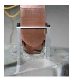
Drill cuts through ice in a laboratory test. Credit: Hong Kong Polytechnic University.
