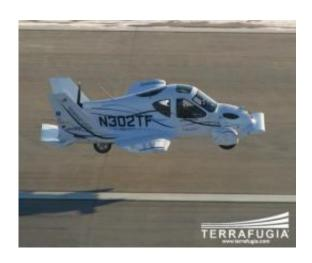
The Terrafugia Transition is a roadable aircraft that was tested last year. DARPA's plans for the Transformer X call for the vehicle to be capable of flying on autopilot and driving off-road, among other features. Credit: Terrafugia.
