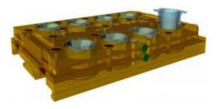
The principle element is the culture plate, in the dimensions of commercially available multiwell plates. Credit: Fraunhofer ITEM
