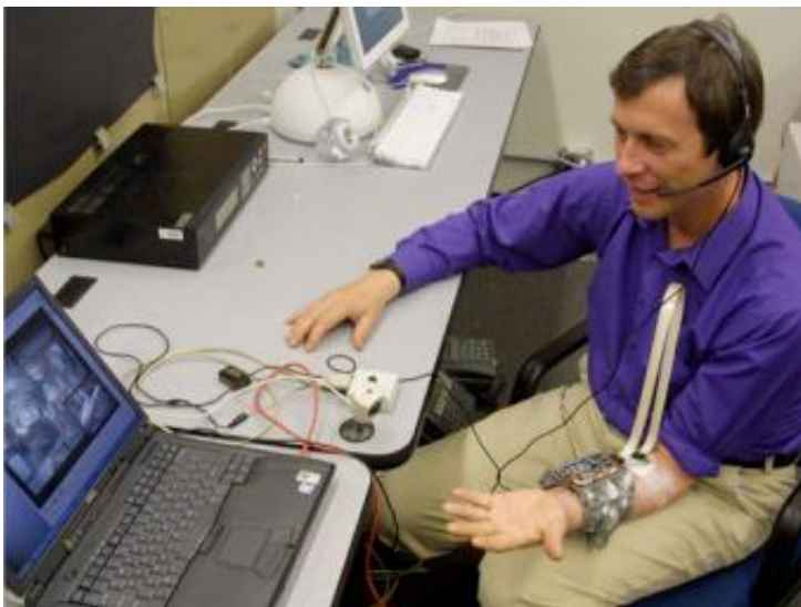
Kevin Warwick with his second cyborg implant. This implant, connected to the median nerve in his arm, allowed him to send and receive signals by computer. Image credit: University of Reading
