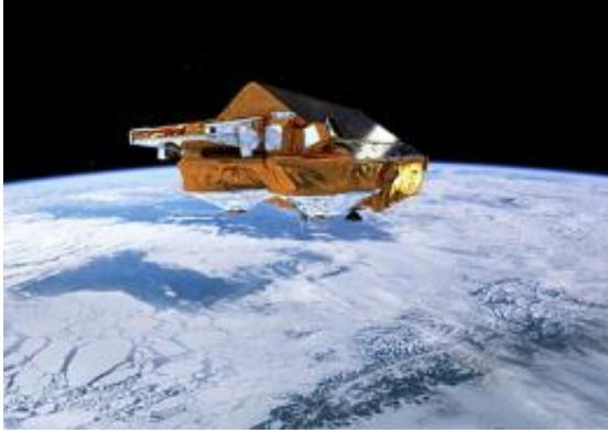
ESA's Earth Explorer CryoSat mission is dedicated to precise monitoring of the changes in the thickness of marine ice floating in the polar oceans and variations in the thickness of the vast ice sheets that overlay Greenland and Antarctica.
