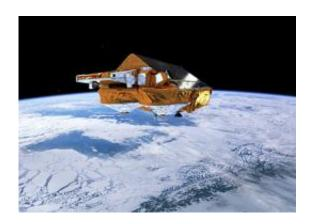
ESA's Earth Explorer CryoSat mission is dedicated to precise monitoring of the changes in the thickness of marine ice floating in the polar oceans and variations in the thickness of the vast ice sheets that overlay Greenland and Antarctica. Credits: ESA - AOES Medialab
